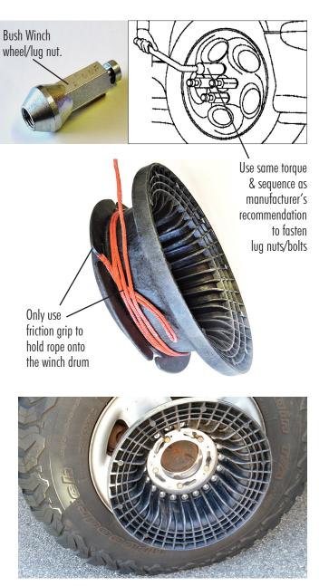
The Bush Winch is suitable for many 4WD's, SUV's and 2WD's, whether front or rear wheel drive. You can go either forward or backwards. All control is from the driver seat and as long as your engine is running, you have ample undiminished power. 7. When screwing on the wheel nuts/lugs or bolts, use the same torque and procedure to tighten them as required for the originals by the manufacturer. It is not necessary to tighten them any harder because the Bush Winch is to be used.
