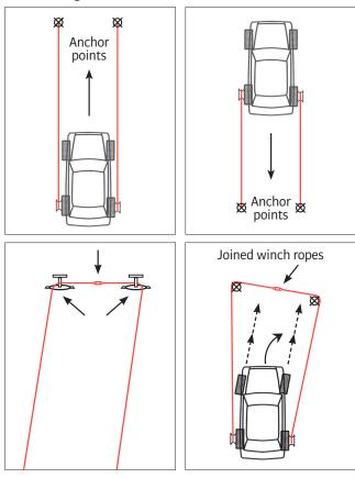
**3.** Using both anchors together **4.** Joined winch ropes. with joined winch ropes.
