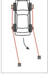
**3.** Going forward around corner with joined winch rope.
